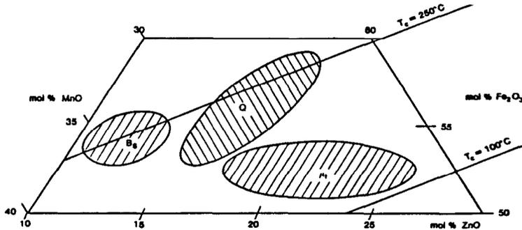
Fig. 2 Triaxial Diagram of Ferrite Compositions
