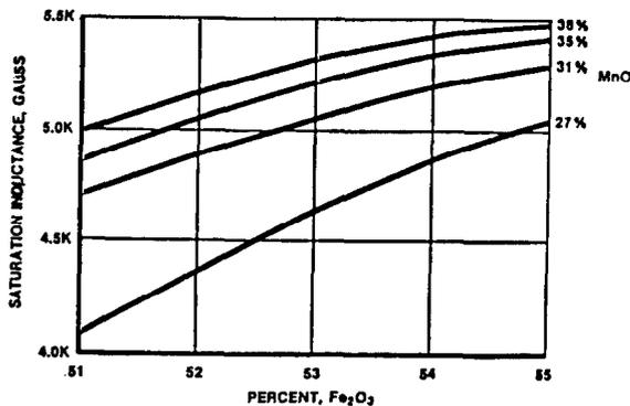
Fig. 3 Saturation Flux Density Versus Composition
