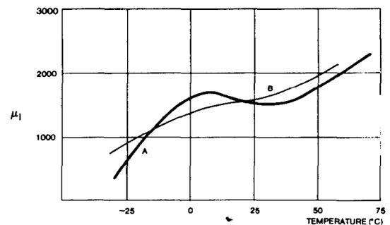
Fig. 6 Core  $\mu$  Versus Temperature
