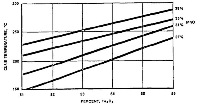
Fig. 4 Curie Temperature Versus Composition
