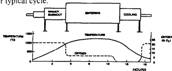
Fig. 8 Typical Firing Cycle
