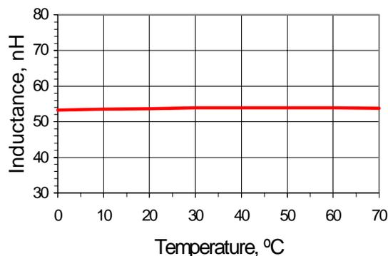
Figure 1 – Typical Temperature Performance
