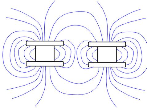
magnetic structure, the Mini-Thick for EMI problems. If two cores are other they will couple and variations (Figure 7). The location and polarity considered. The addition of a ferrite
