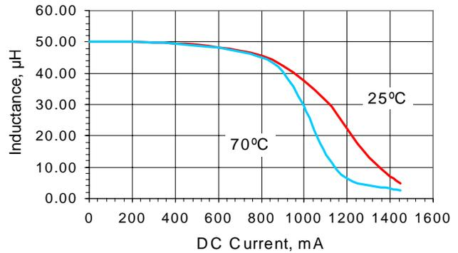
**Figure 4 - Incremental Inductance vs. DC Bias**
