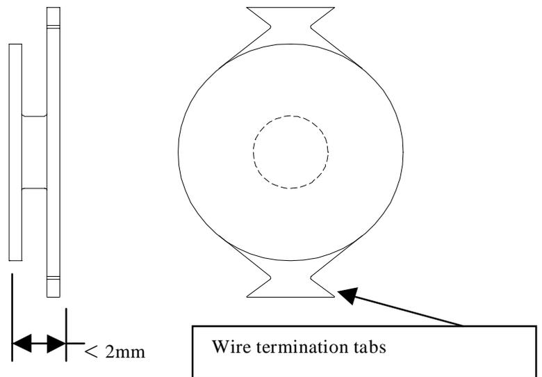
**Figure 5 – The Mini-Thick Bobbin**
